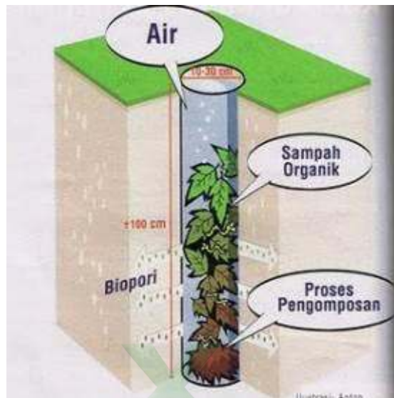
Gambar 2. Gambaran Lubang Biopori
